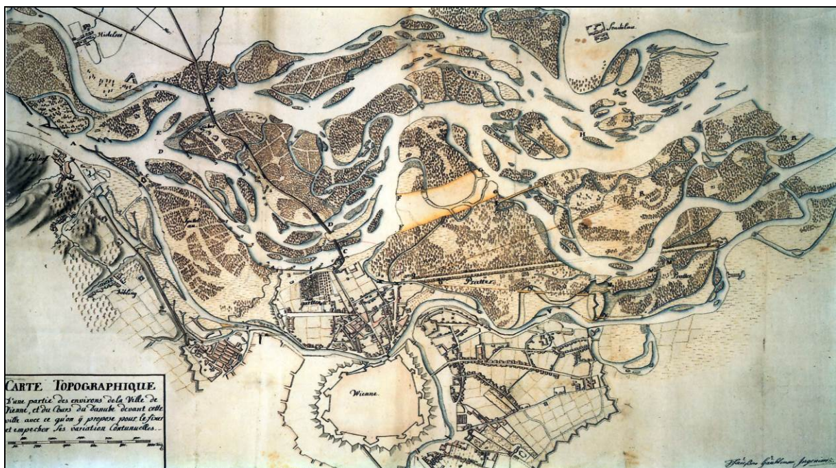
Figure 2: Regulation plan designed by Ritter v. Spal(l)art in 1760; the proposed cut-off channel between two major river arms to improve the Danube's flood conveyance is depicted in the middle of the plan (see footnote 6).
